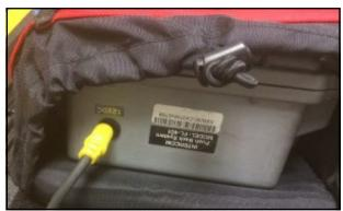
Plug the yellow headset charging cable into the "12VDC" port on the end of the ComHub.
