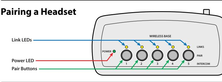
**A.** Press and hold the desired pairing button on your Base Station until its link indicator flashes slowly.
