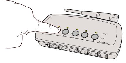
**B.** Starting with your Flightcom Headset turned off, place the Flightcom Headset into pairing mode by pressing the Power and PTT buttons simultaneously until you hear "Base Station registering", then release the Power and PTT buttons.
