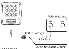
Vehicle Charging Note: Make fuse no further than 18" from the battery. Note: Only replace fuse with the same type, 1.5A AGU.
