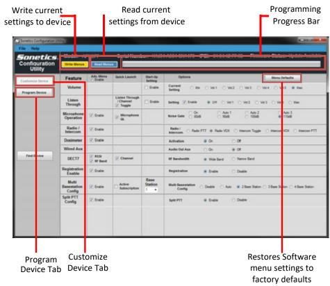
The **Program Device** tab presents information about the device's current firmware version, and allows you to update the device's firmware if required.
